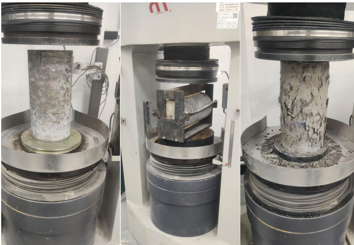
**Fig. 5** Compressive strength test setup on PAC and FR-PAC samples
