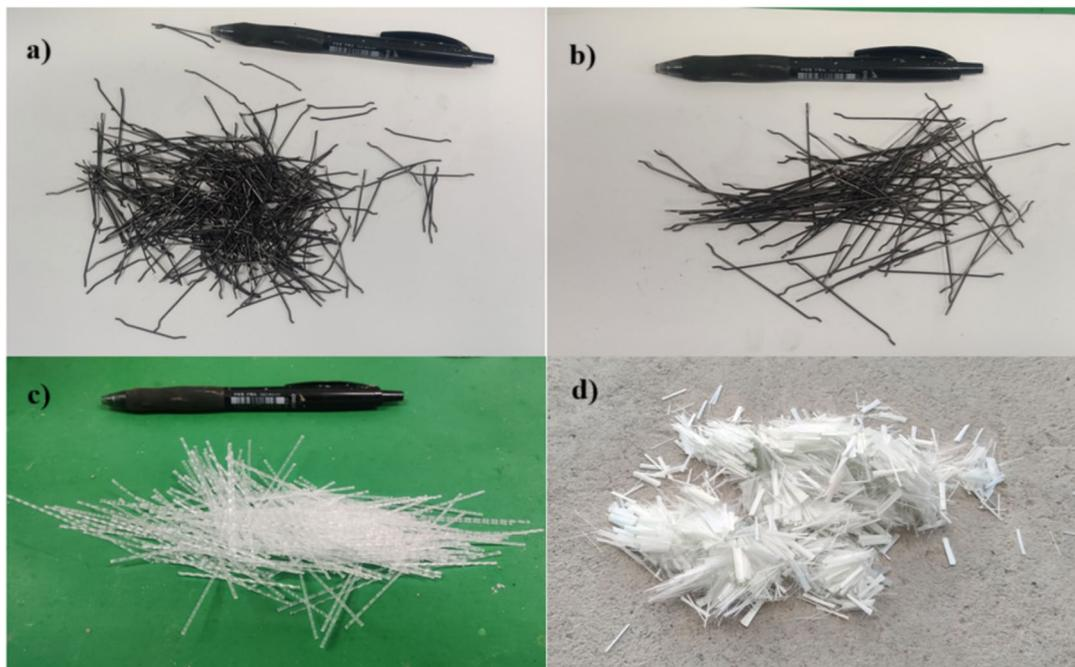
**Fig. 2** Types of fibers used in this study: **a** short hooked-end steel fibers, **b** long hooked-end steel fibers, **c** polypropylene fibers, and **d** glass fibers
