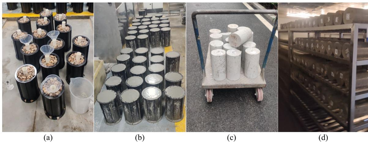
**Fig. 3** PAC's mixing procedure, **a** positioning coarse aggregates by injection tubes in cylinder molds above shaker machine; **b** PAC mixtures after grout injection; **c** molded specimens; and **d** curing of specimens in curing room
