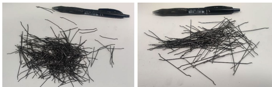
Figure 4. Short hooked end steel fibers (Left) and long hooked end steel fibers (right).
