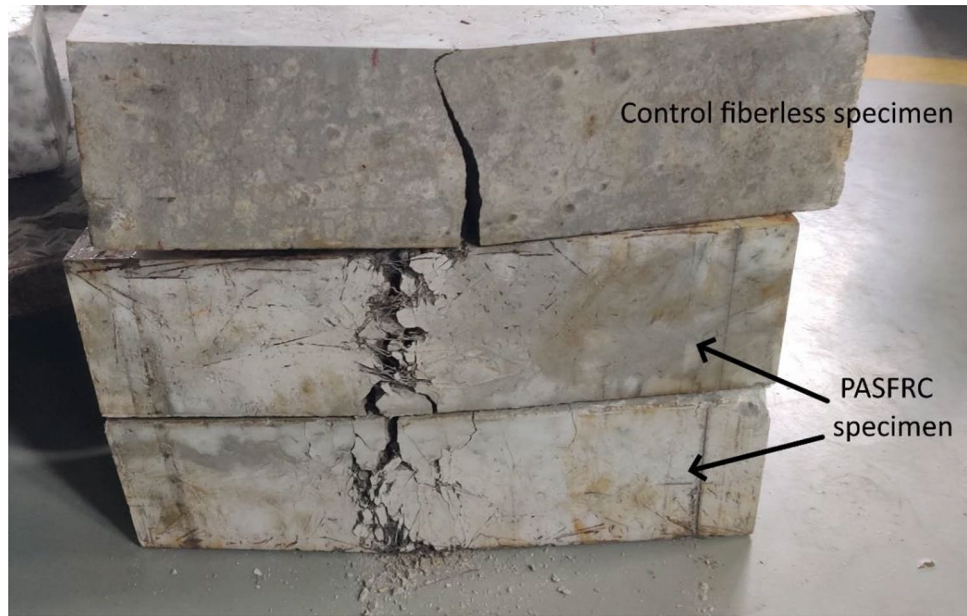
Figure 12. Flexural failure mode of both fiberless and steel reinforced PASFRC specimens.
