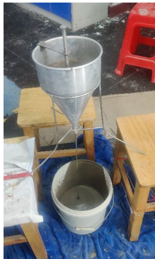
Figure 2. Determining the efflux time using the flow cone test.
