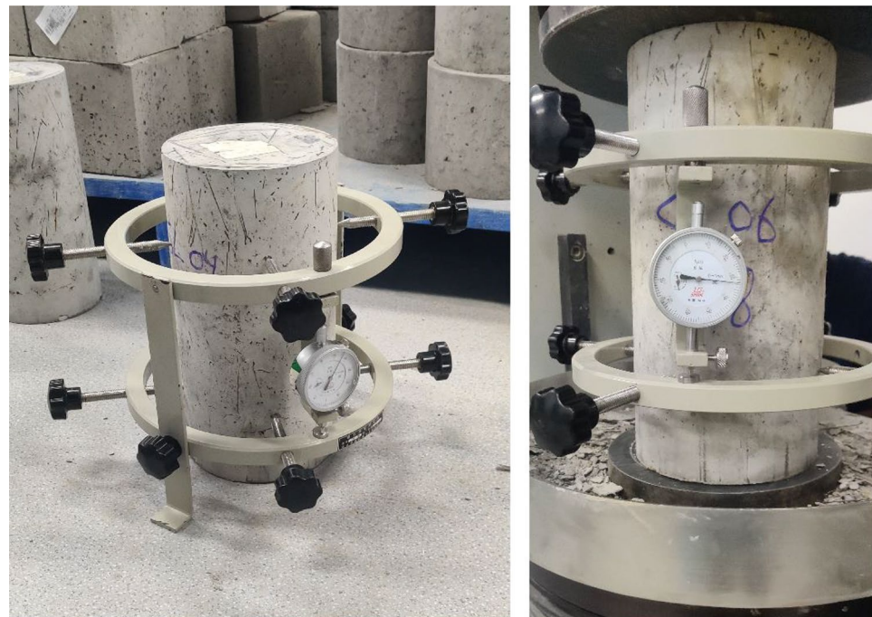
Figure 6. Modulus of elasticity test setup.
